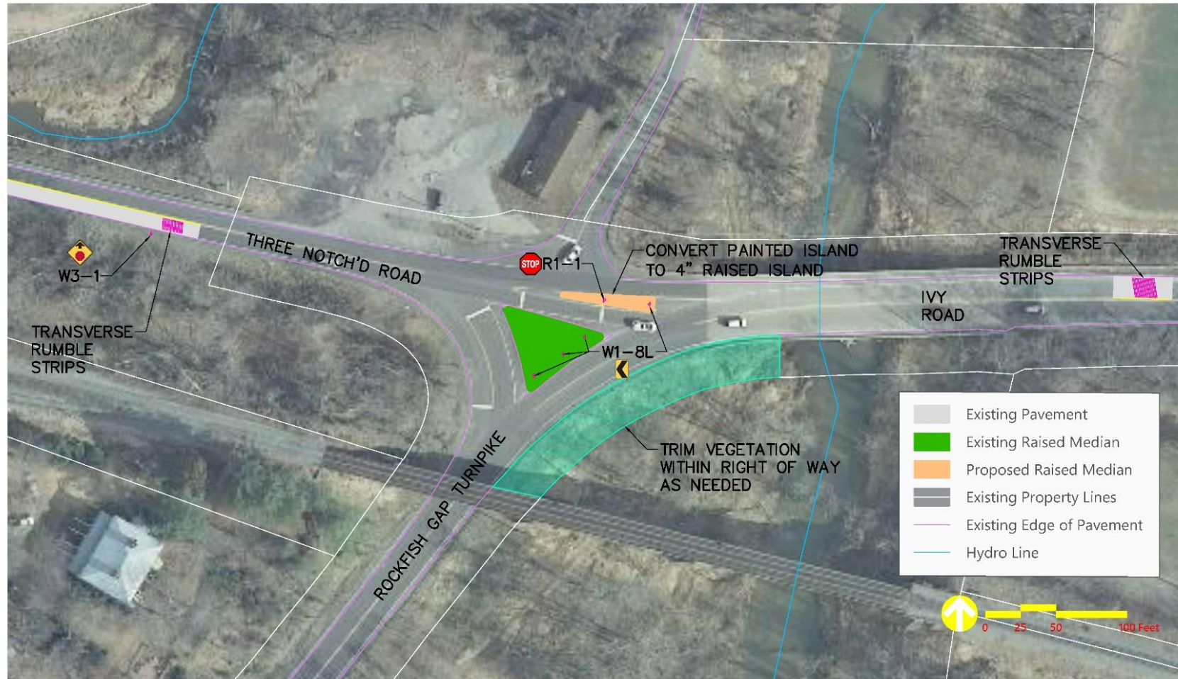
Figure 7.9 – Short-Term Concept for Ivy Road / Rockfish Gap Turnpike and Three Notch'd Road
