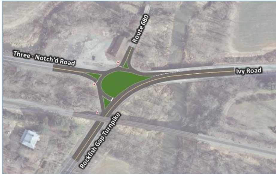
Figure 7.4 – Partial Roundabout, Stop Controlled Concept
