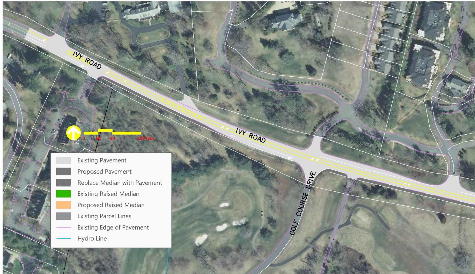
Figure 7.66 – Four-Lane Widening Concept (A) for Ivy Road
