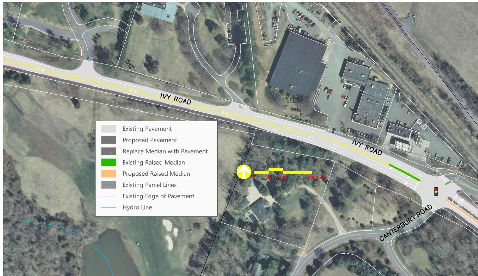
Figure 7.65 – Four-Lane Widening Concept (A) for Ivy Road
