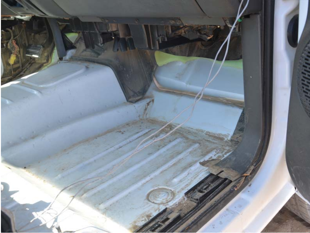
FIGURE 59. Post-Test View of Passenger's Floorpan
