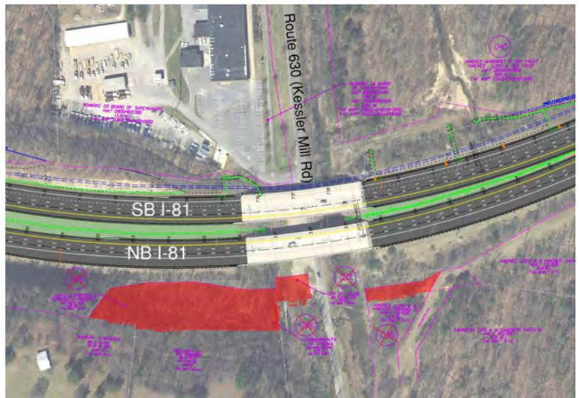
Figure 4.3.3 – Proposed right-of-way acquisitions adjacent to northbound I-81 have been eliminated (as indicated with red shading) due to the elimination of the stormwater management pond immediately south of Kessler Mill Road
