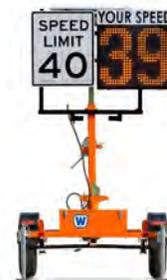
Figure 4.5.15 - Speed display/radar trailer
