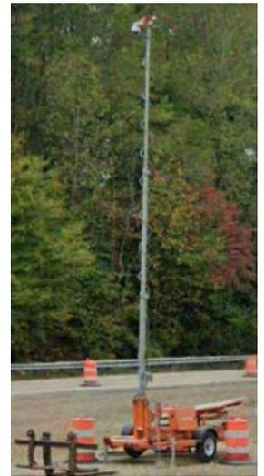
Figure 4.5.18 - Portable CCTV unit
