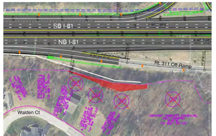
Figure 4.3.5 –By shifting Noise Barrier IK slightly to be located within existing right-of-way, impacts to four (4) properties have been eliminated
